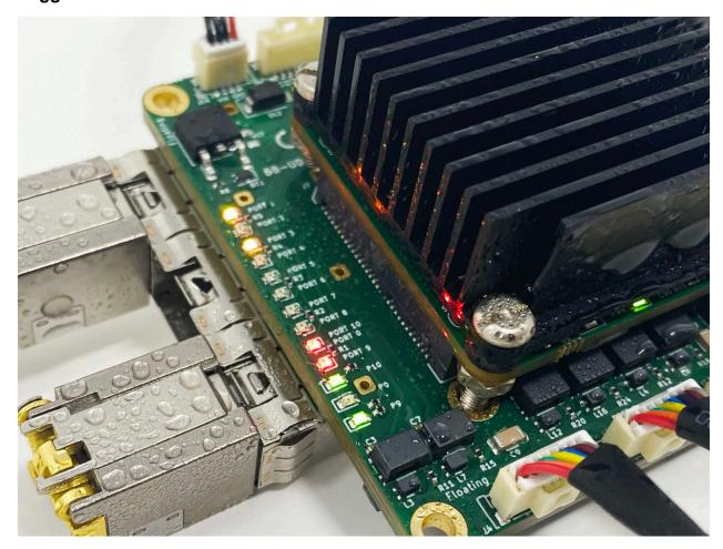
UbiSwitch is tested for operation between -70 to +110°C, which makes it highly optimized for tough environments. This temperature range is achieved using automotive and military-grade parts and fully tested to MIL-STD-810H standard (these test results are fully available).
