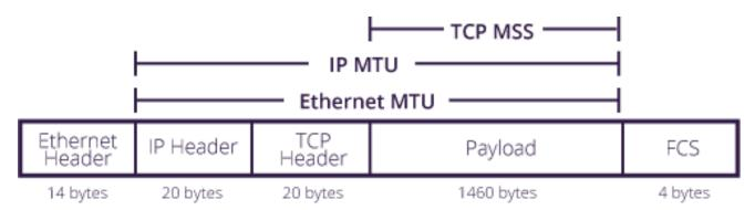
A small MTU is beneficial because it reduces the chance of an error causing frame corruption ; essentially, less time on the wire means less likelihood of bit errors). However small MTUs mean that less of the bits actually sent are payload, meaning reduced efficiency and reduced overall data rate. For this reason, many GigE Vision cameras are designed to support an MTU larger than 1500 bytes, the most common being 9000 bytes (called Jumbo Frames).
