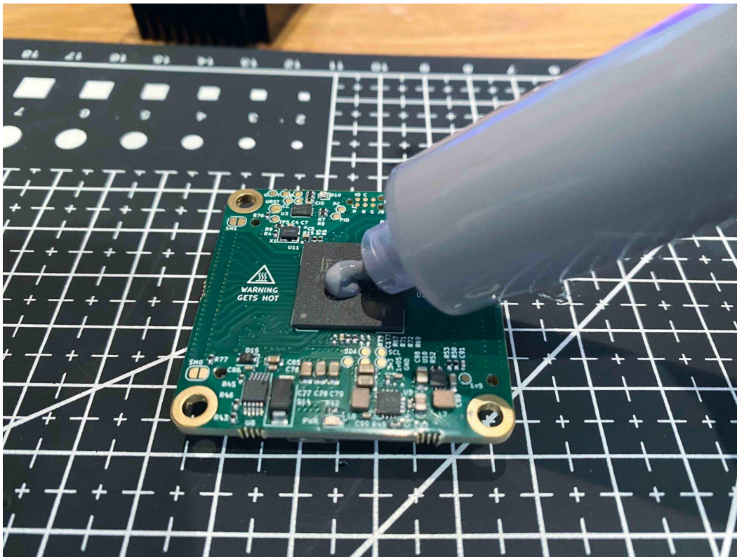
Figure 12. Applying thermal paste to UbiSwitch
