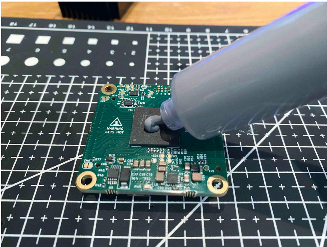
Figure 12. Applying thermal paste to UbiSwitch
