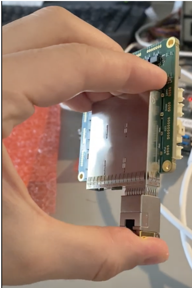
Figure 9: How to insert an SFP into the SFP cage without risking damage to any components on the board.
