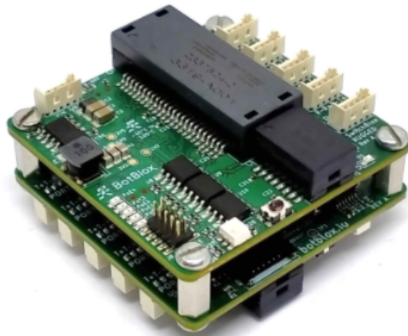
Figure 13: Back to Back operation (two SwitchBlox Rugged)
