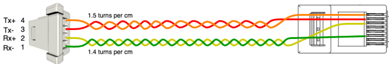
Figure 11: Ethernet cable pinout for Molex PicoClasp variant
