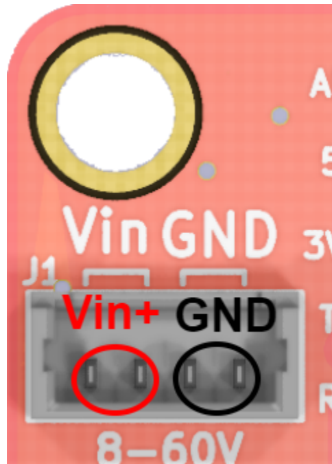
Figure 4: Voltage input header pinout
