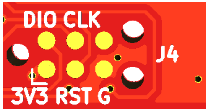
Figure 10: SWD programming header pinout
