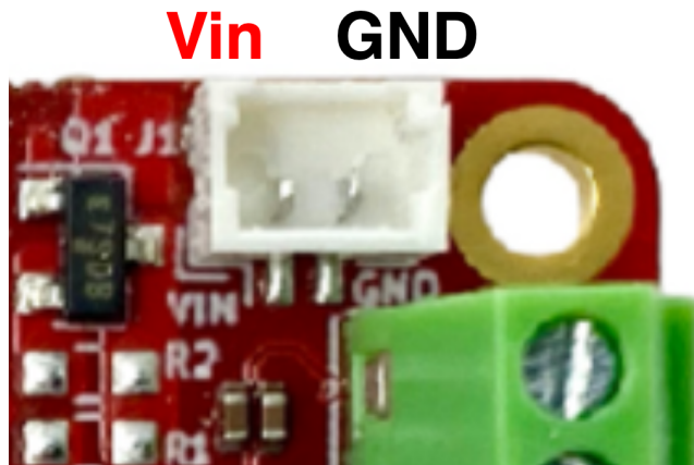
Figure 5: Voltage input header pinout
