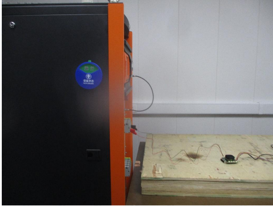
Fig.24 Electrical fast transient/burst immunity signal port set-up
