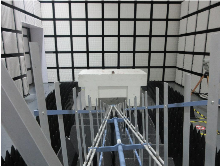
Fig.14 Radiated emissions 1 GHz ~ 6 GHz test set-up
