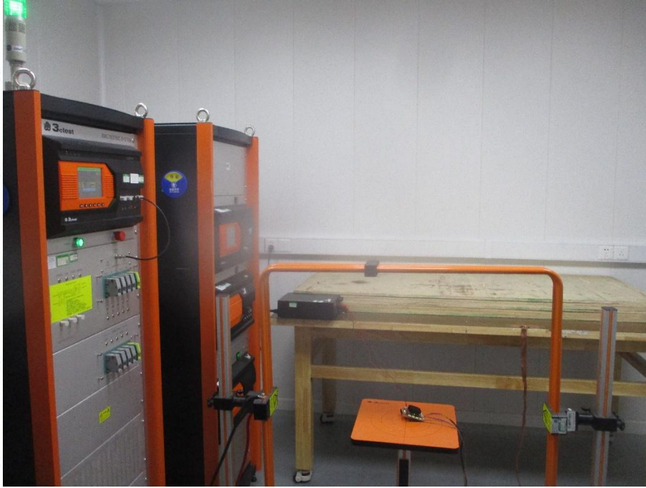
Fig.26 Power frequency magnetic field test set-up
