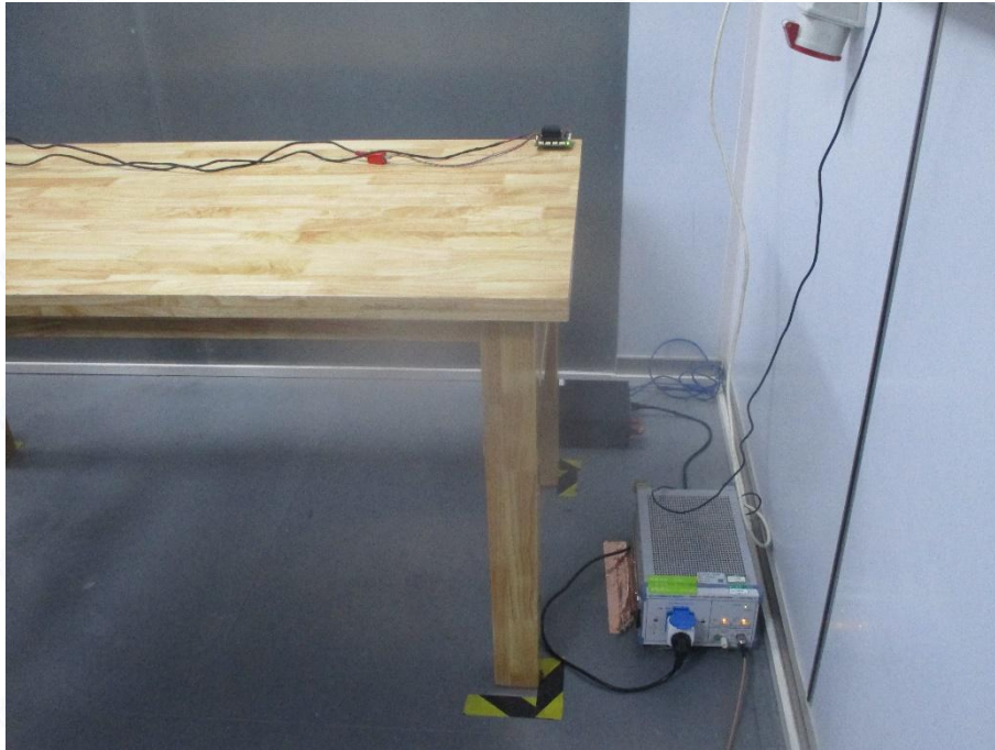
Fig.5 Conducted emissions from the power ports test set-up
