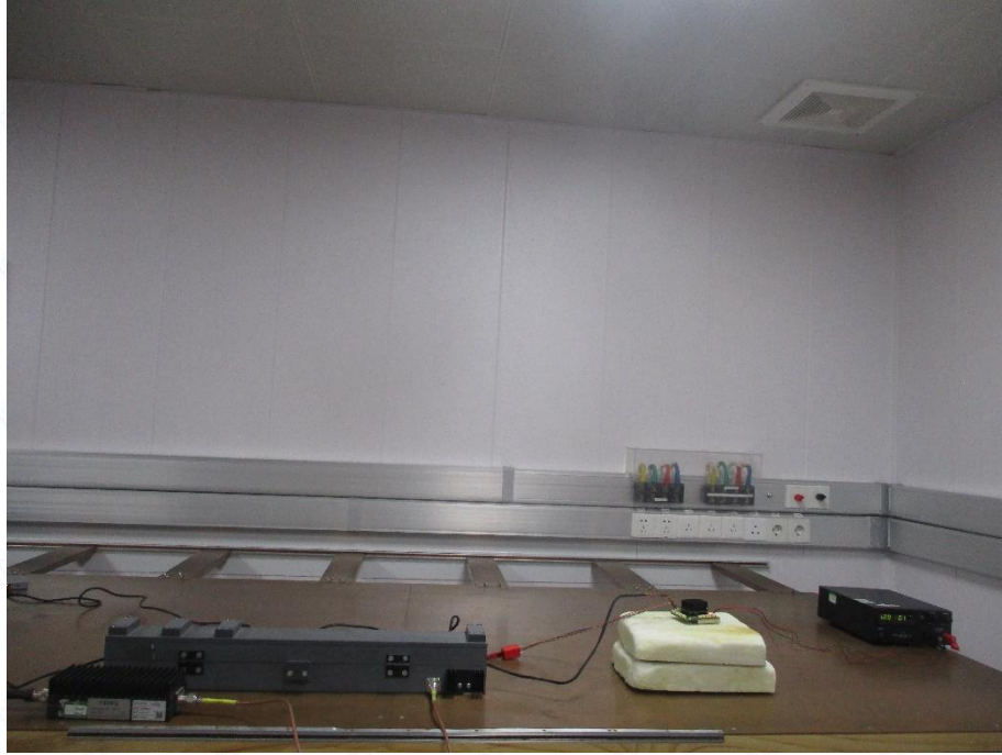
Fig.25 Immunity to conducted disturbance, induced by radio-frequency fields test set-up
