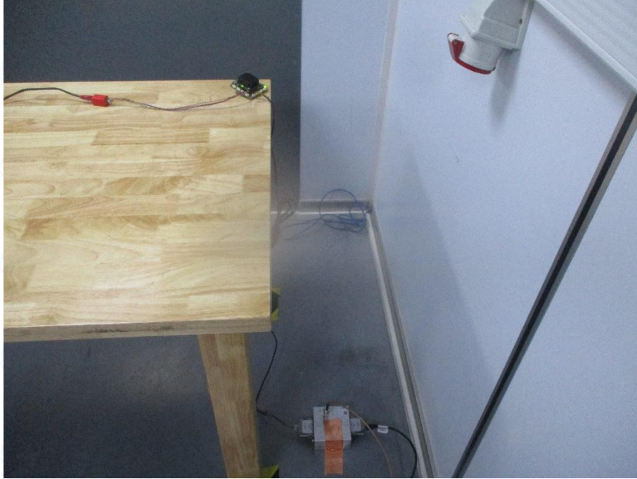
Fig.10 Conducted emissions from the signal ports test set-up
