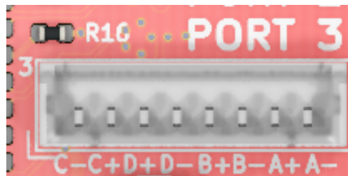
Figure 2: Mapping of ethernet signals onto PicoBlade connectors.
