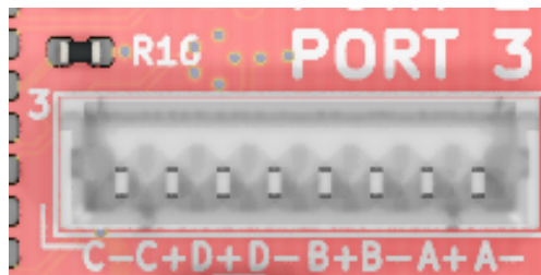
Figure 7: Mapping of ethernet signals onto PicoBlade connectors.
