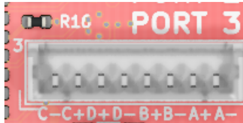
Figure 7: Mapping of ethernet signals onto PicoBlade connectors.
