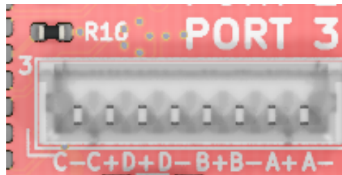
Figure 6: Ethernet port pinout
